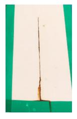
790 hrs salt spray exposure DFT = 50-60 microns over SA 2.5 blasted steel panels
