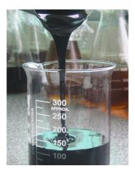
CNSL resins are used as a binder for friction products such as brake pads, linings and blocks. Together with hexamine as cross-linking agent, they provide a heat curable thermosetting system that offers the desirable characteristics of impact resistance, flexibility and thermal stability. Cardolite offers a wide range of liquid binder resins, including high and low viscosities, solvent-free, solvent cut and elastomer modified grades.
